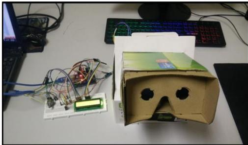
Figure 2: Arduino based CFF device
